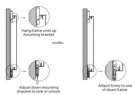
For uninstall of screen, unscrew down mounting brackets till it is loosen from slot of down frame. Lift the screen lightly to make it go off upper mounting bracket and finish uninstall.
