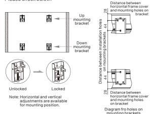
Please make sure the brackets are firmly installed. Hang the screen onto upper mounting bracket and make adjustment until upper bracket is at the middle of screen. Let the screen hanged vertically and tight the screw of down mounting bracket until screw is attached to slot of down frame. Please check below:
