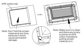
Use the bigger hook of spring to hitch tension rod from the hole of screen material one by one. Use hook hand to drag the small hook of spring to hitch the slot of frame to tension the screen material.
